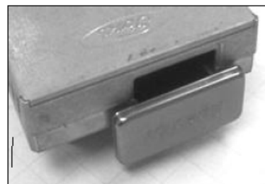
Fig 6 -Chip incorrectly mounted
